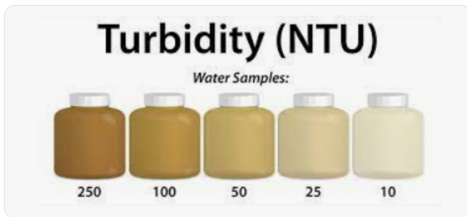
Turbidity colour chart and average turbidity range.
