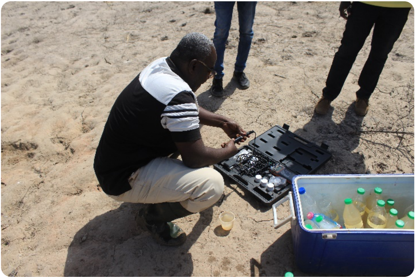
Abdul-Latif Salifu (Chief Technical Officer) from the Water Research Institute (WRI) running real-time water quality testing using a Multiparameter Water Quality Meter.
